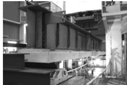
Fig.2 Negative bending test for intermediate support of continuous girder
