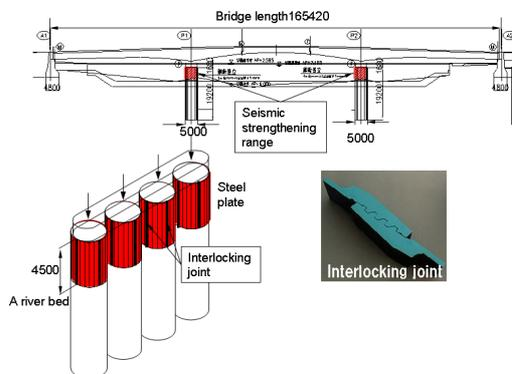
Fig.1 Seismic strengthening outlines
