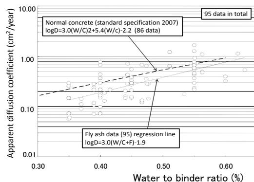
Fig.3 Apparent chloride diffusion coefficient
