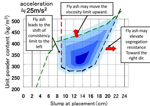
Fig.2 Limit-state boundary of workability
