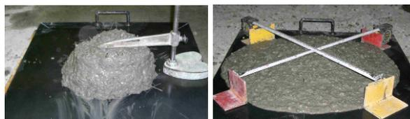
Ordinal concrete (Slump 15±2.5cm) Middle fluidity concrete (Slump flow 35-50cm)
