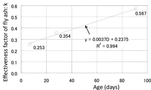
Fig.1 Effective ratio of fly ash on strength
