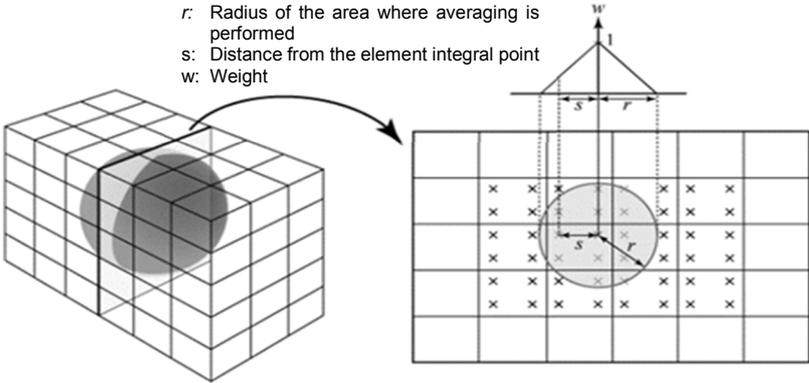
**Fig-4.1: Schematic View of Weighted Averaging of Local Damage Indicators<sup>4)</sup>**
