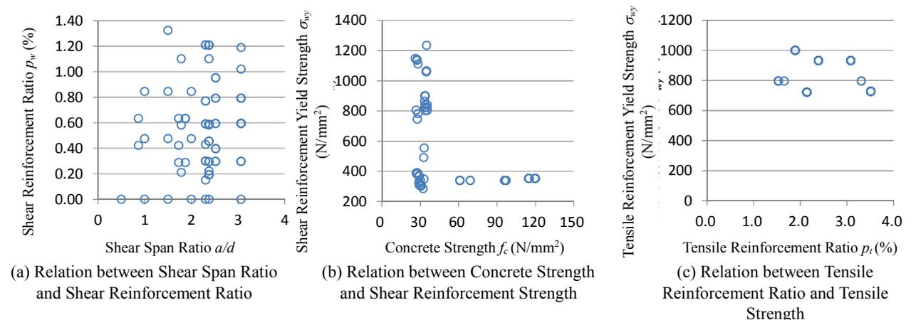
**Fig.-3.1: Experimental Data Used for Establishing Macro Formulas (Beams)**
