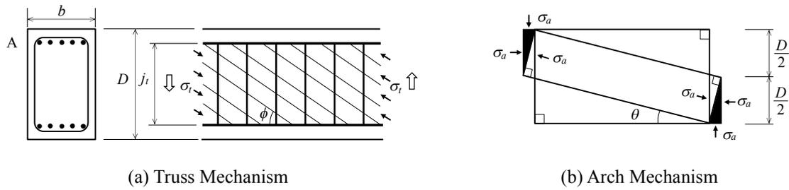
**Fig.-3.2: Shear Resistance Mechanism in the 1990 AIJ Guidelines for Reinforced Concrete Buildings**
