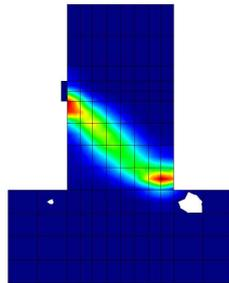
**Fig.-4.2: Example of Distribution of Normalized Cumulative Strain Energy of Wall Member Subjected to Horizontal Force**
