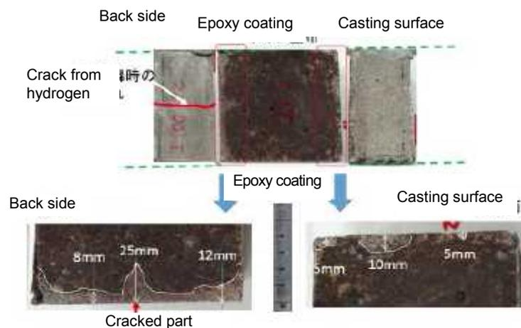
**Fig. 2.3: Salt permeation in a test piece (with a crack)**
