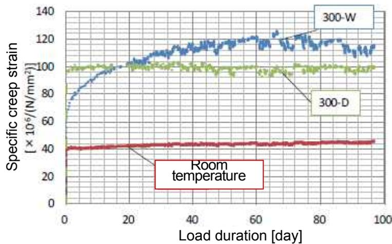
**Fig. 2.4:** Change in specific creep strain [4]
