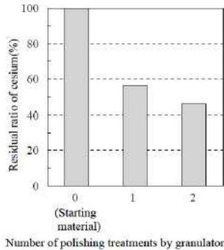
**Fig. 3.1: Change in the Cs residual rate of mock contaminated concrete piece crushed by granulator**
