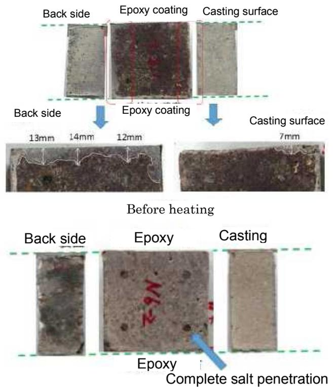
After 500°C heating (complete penetration)
