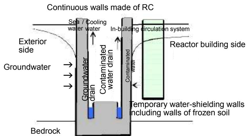
**Fig. 2.8: Underground double reinforced concrete (RC) continuous walls assumed to shield water for 300 years**
