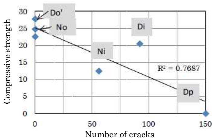
**Fig. 2.2: Relation between the number of cracks and compressive strength [2]**
