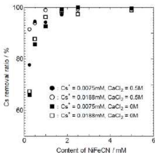
**Fig. 3.2: Effect of NiFeCN concentration on Cs decontamination performance [22]**
