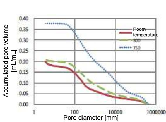
**Fig. 2.5: Change in pore volume by heating [4]**
