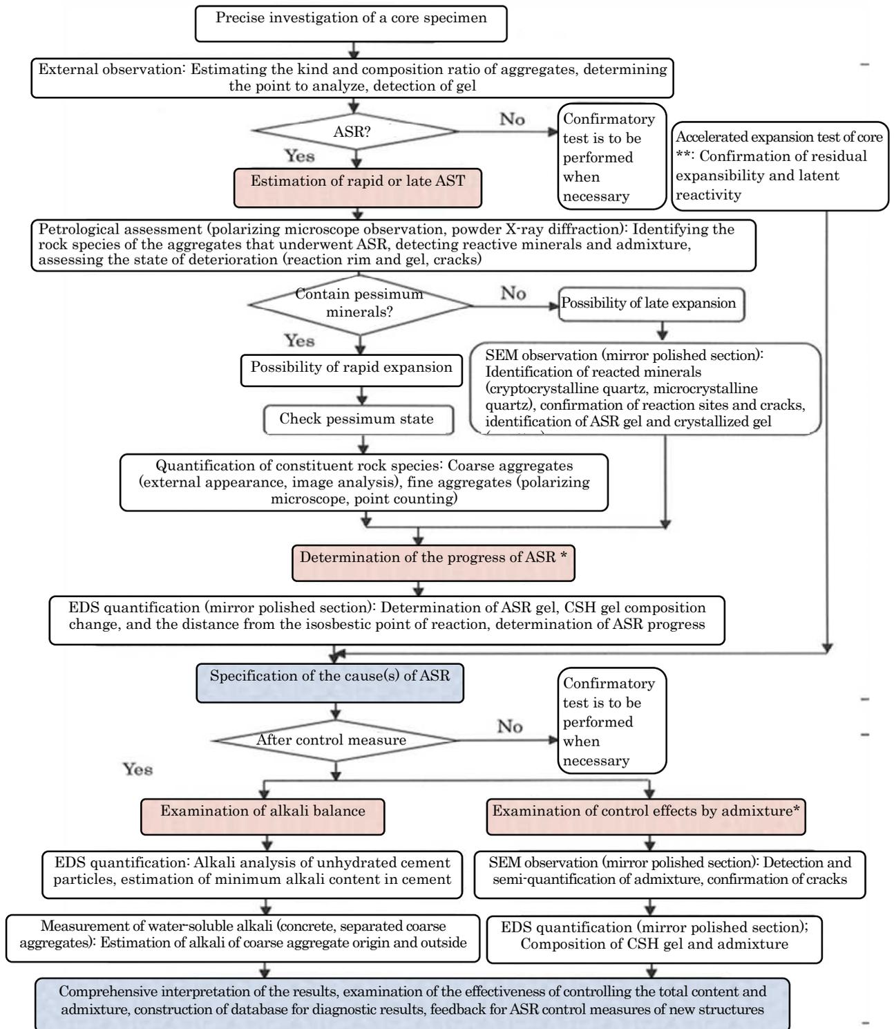
Fig. 2.2 (cont.) ASR diagnosis flow for concrete structures (draft)
