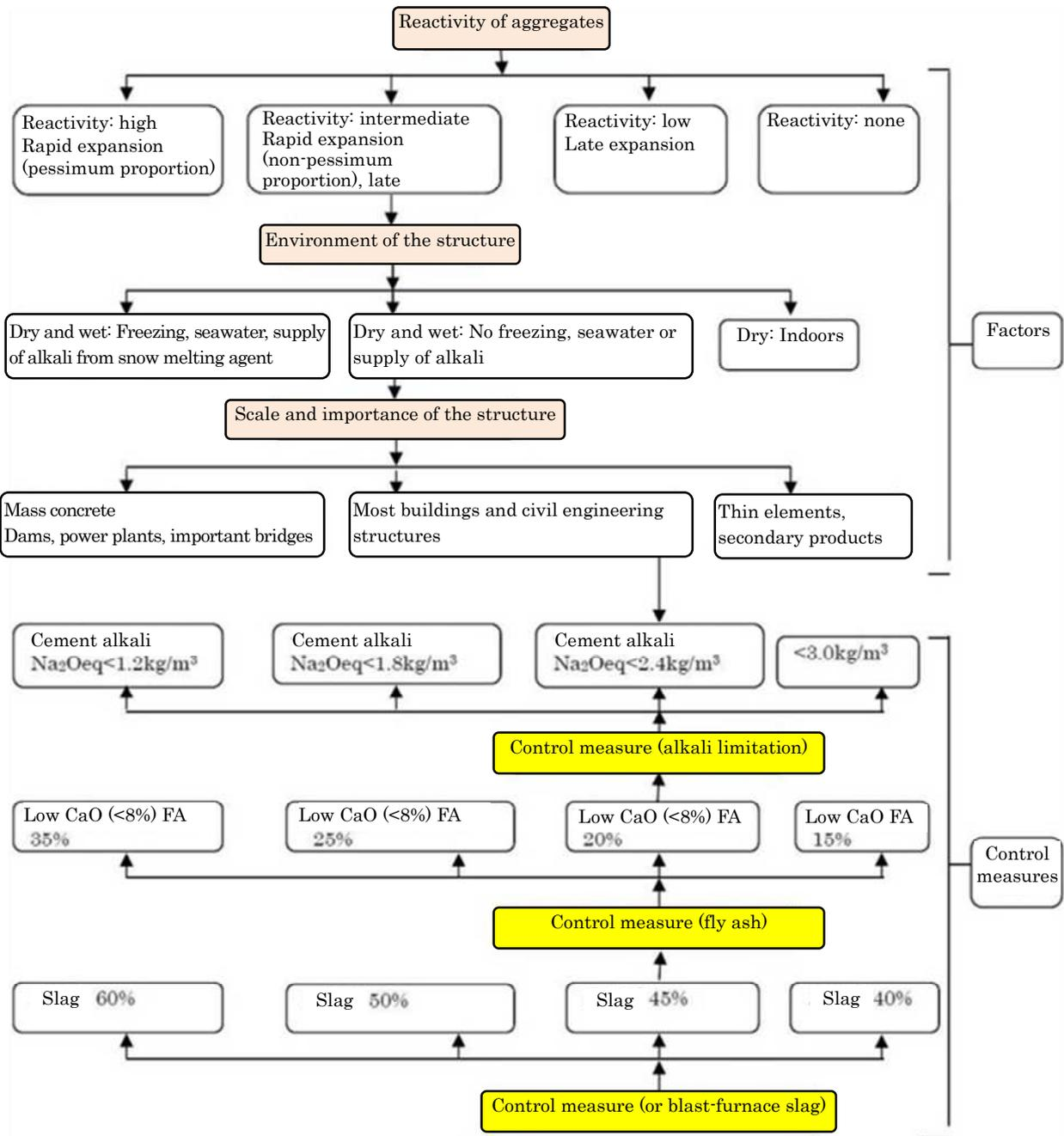
Fig. 3: Flow of selecting control measures <sup>6)</sup>
