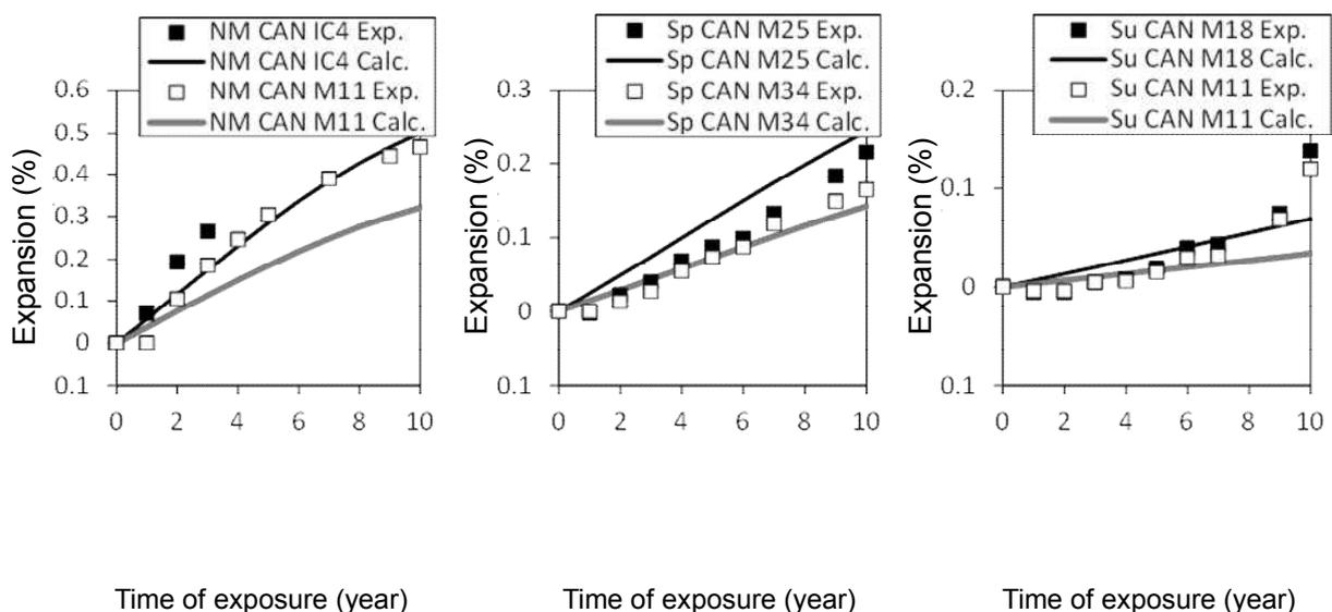
**Fig. 5: Example of simple expansion prediction using CPT<sup>8)</sup>**
