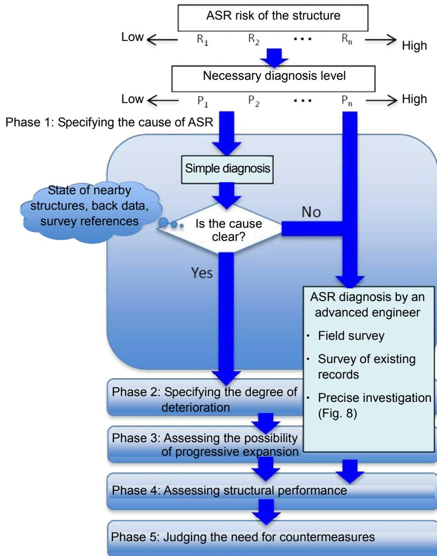
**Fig. 7: Framework of ASR diagnostic flow**
