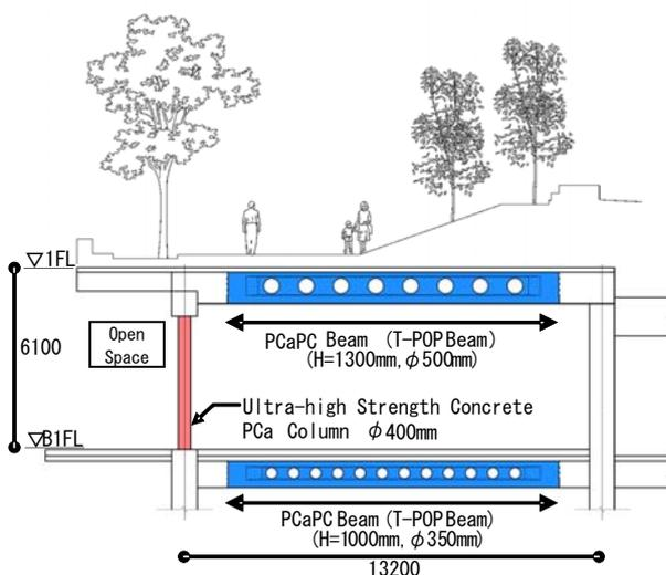
Fig.2 General Structural Framing details below artificial ground
