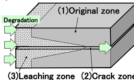
If cementitious materials are used as a barrier component, the influence of **leaching** and **crack generation** must be considered.
