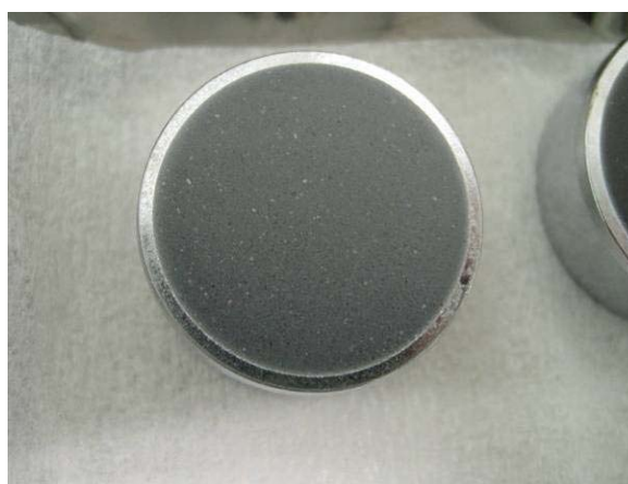
Photo.1 Press-formed Sample ( d = 35 mm)
