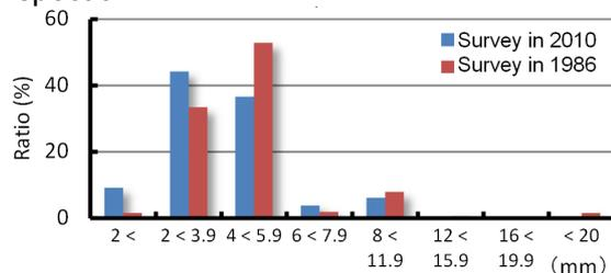
Fig.3 Target value of formwork (street accuracy at the top of formwork)
