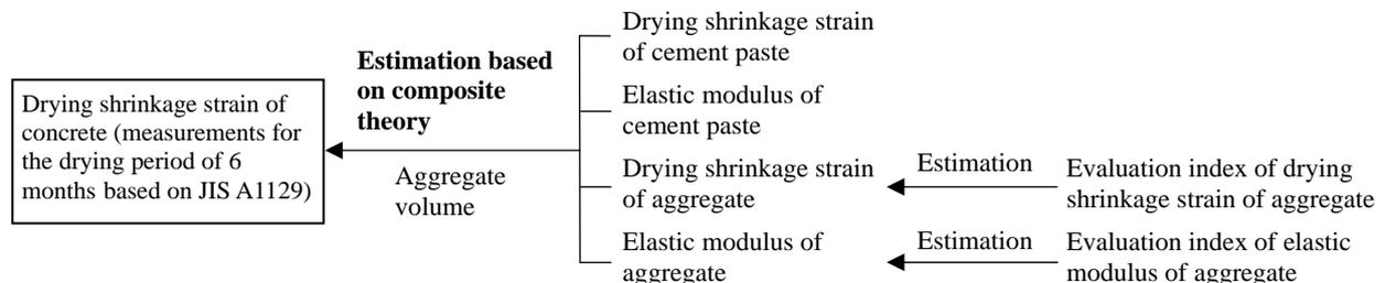
Fig. 1 Estimation Flow of Drying Shrinkage Strain of Concrete
