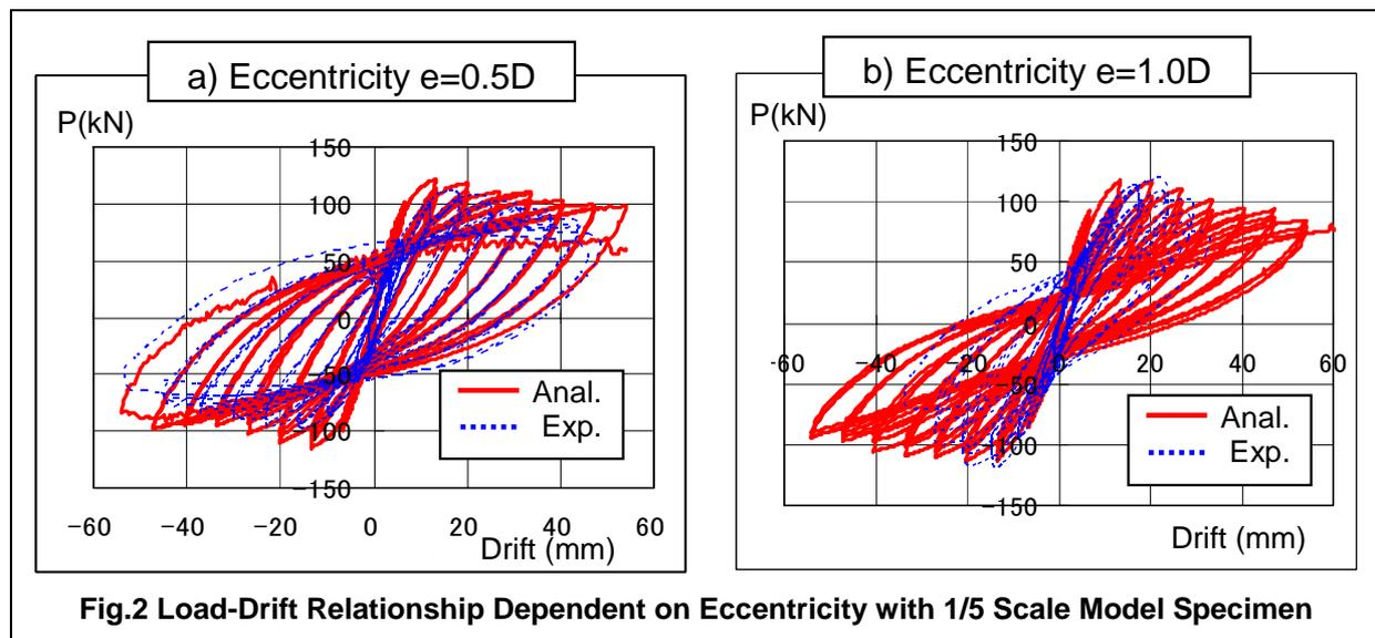
**Fig.2 Load-Drift Relationship Dependent on Eccentricity with 1/5 Scale Model Specimen**
