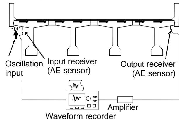
Fig. 1 Impact elastic-wave method
