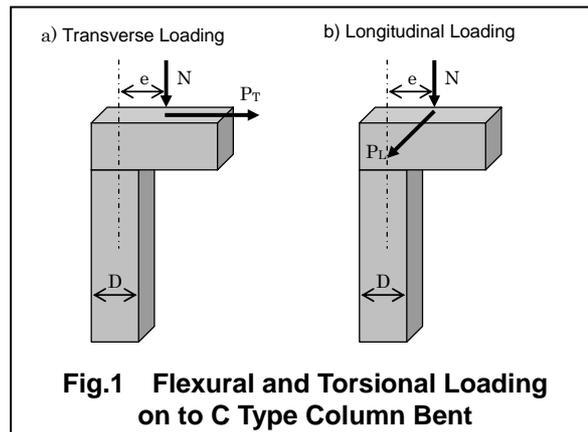
**Fig.1 Flexural and Torsional Loading on to C Type Column Bent**
