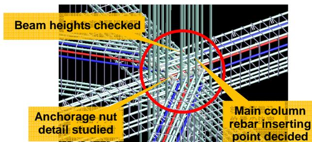
Fig.2 Rebar detailing study: Connection of diagonal beams to PC sub-beams
