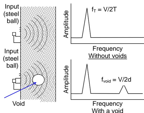
Fig. 2 Frequency response characteristics with and without voids
