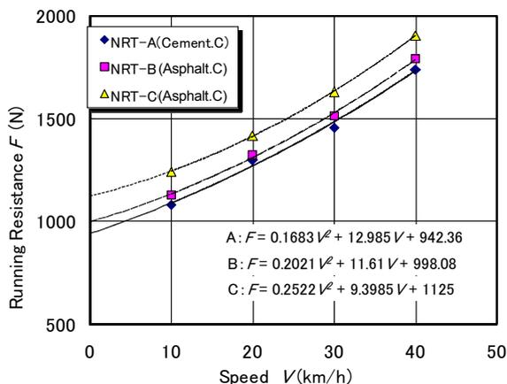
Fig.1 Result of running resistance at the NRT
