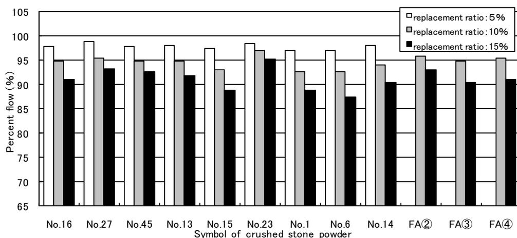
Fig.1 Percent flow of mortar with equivalent slump 8cm, W/C=0.55, crushed sand (normal)
