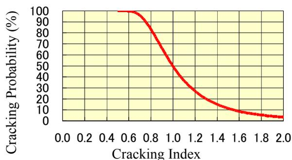
Fig. 1 Suggested Cracking Probability Curve
