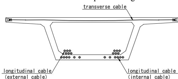
Figure-1 General cross section of box girder and example of placement of PC cables.
