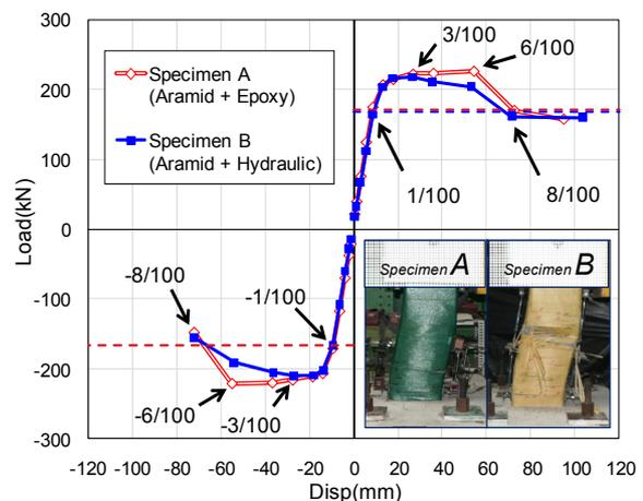
Fig. 1 Load-displacement curve and the failure conditions
