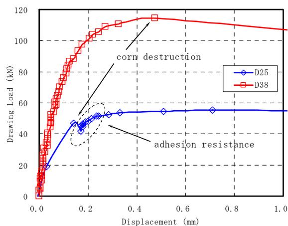
Fig.1 Load – displacement relations
