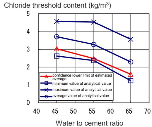
Fig.2 Threshold chloride content to water-cement ratio
