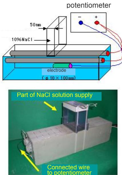
Fig.1 Monitoring method of half-cell potential
