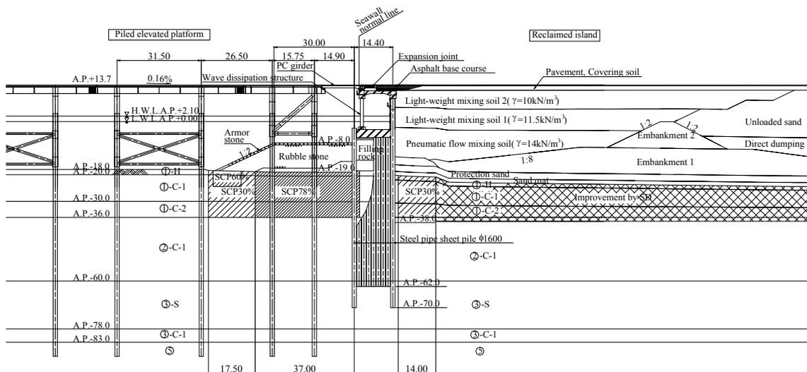
Fig.1 Cross section of steel pipe sheet-pile cellular seawall
