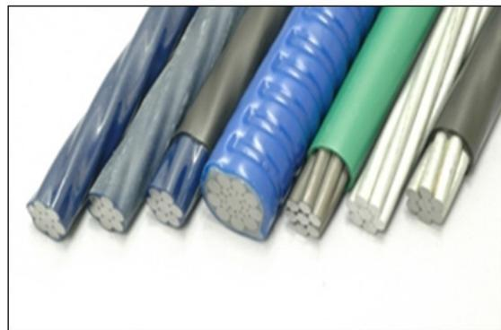
**Photo-1** Variety of factory applied corrosion protection (from left to right, ECF strand (smooth), ECF strand (grit impregnated), HDPE extruded ECF strand, EPG strand, unbonded strand (greased and HDPE extruded), galvanized strand, galvanized and wax filled HDPE extruded )
