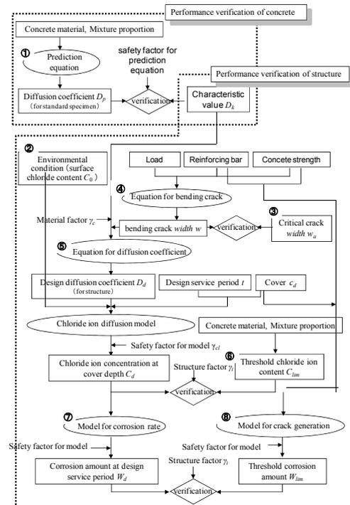
Fig.3 Performance verification on chloride attack
