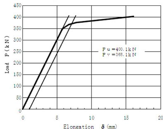
**Fig-1** Example of load-elongation curve of 2230MPa grade high-strength strand under cryogenic condition(-196°C)
