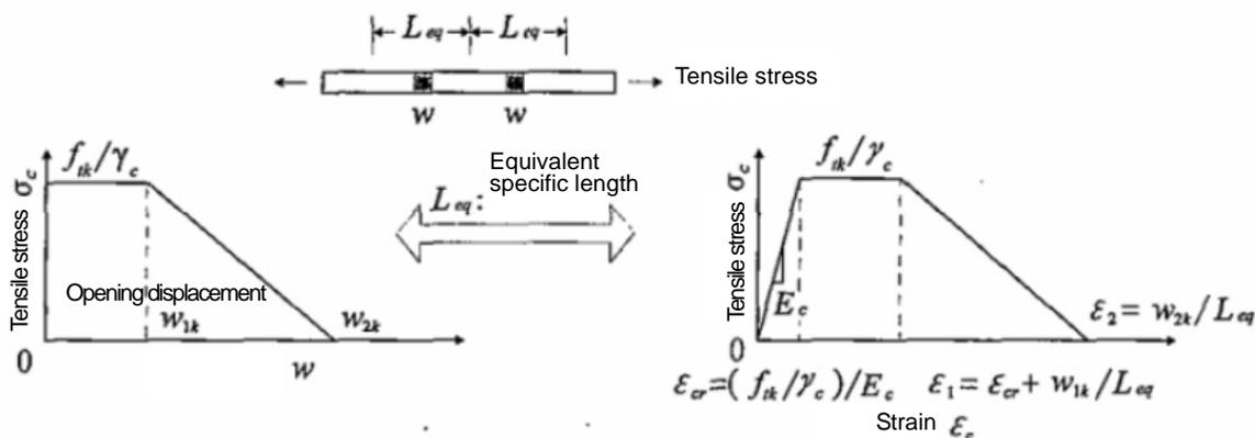
Fig. 3: Relationship between tension softening diagram and tensile stress-strain curve<sup>6)</sup>
