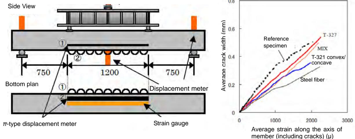
**Fig. 6: Evaluation of average crack width of different fiber-mixed ferroconcrete members**<sup>13)</sup>
