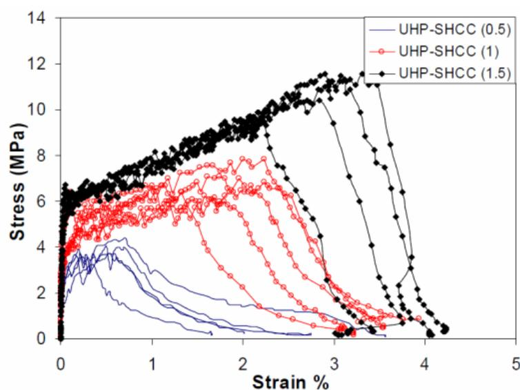
**Fig. 4: UHP-SHCC tensile stress-strain relationship<sup>7)</sup>**
