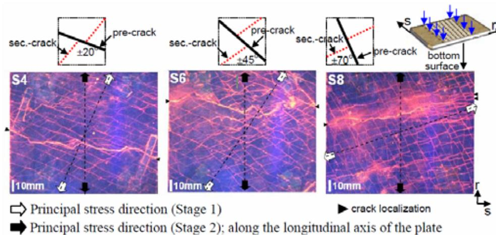
**Fig. 8: Multidirectional cracking due to revolution of principal stress axis<sup>16)</sup>**
