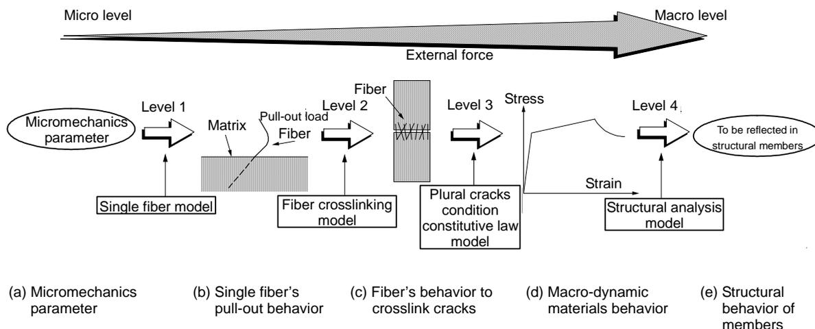
Fig. 2: Materials design technology for ECC<sup>5)</sup>
