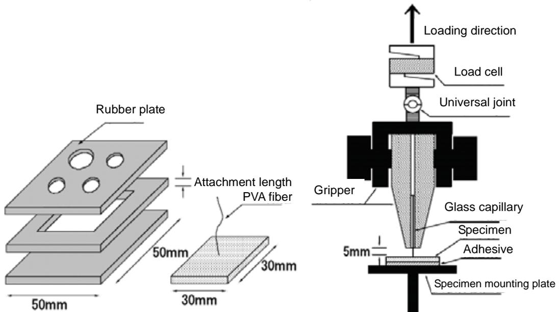
Fig. 10: Single fiber attachment test method<sup>18)</sup>
