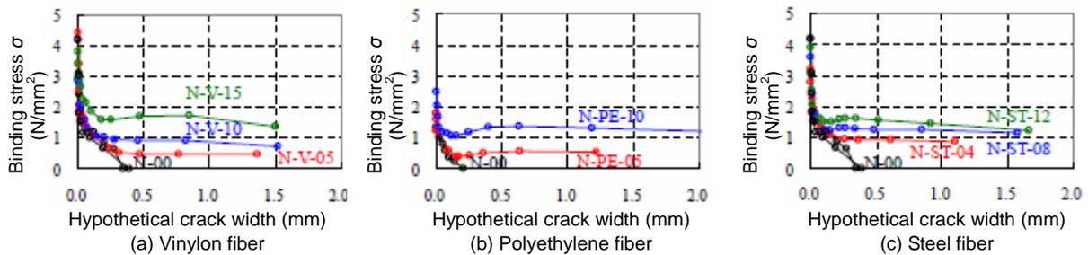
**Fig. 5: Different fiber-mixed concrete tension softening diagram comparison**<sup>12)</sup>
