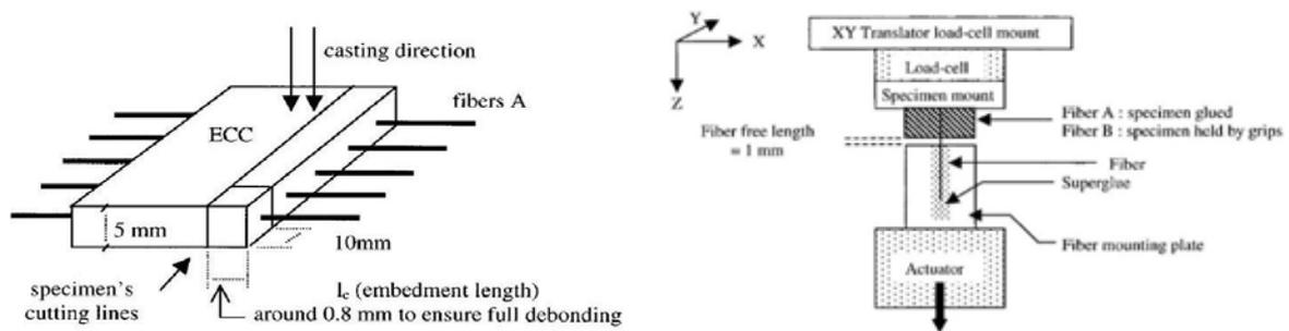
Fig. 9: Single fiber attachment test method<sup>17)</sup>
